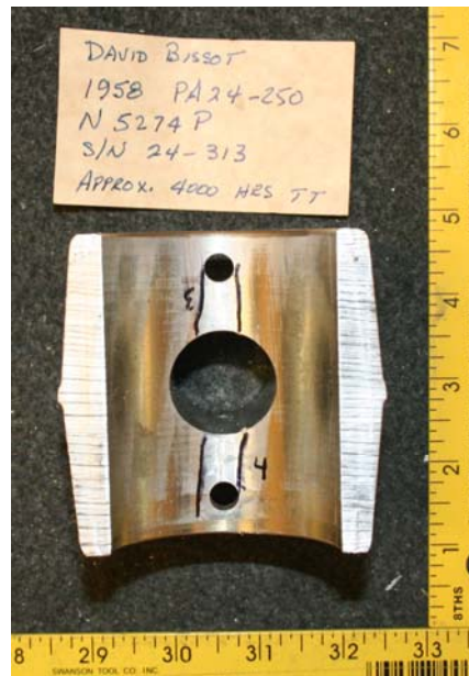
Figure 23 – Surface A of the Large Diameter Bore from A/C N5274P
