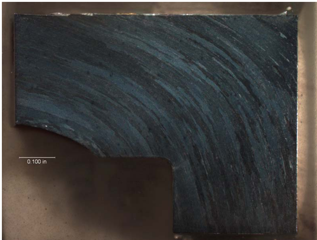
Figure 33 – Grain Flow Pattern from A/C N7545P
