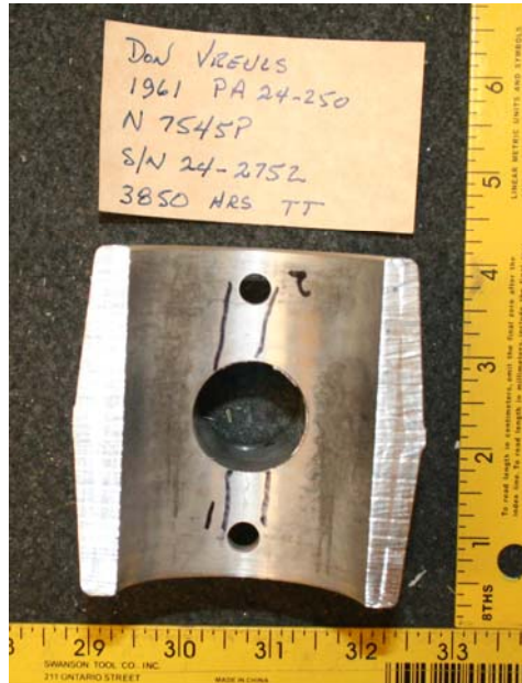
Figure 22 – Surface A of the Large Diameter Bore from A/C N7545P
