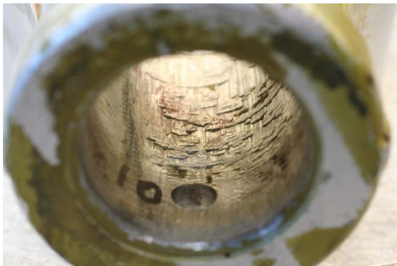
Figure 20 – Smeared Metal on Surface B from A/C N7545P
